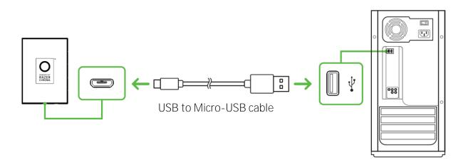
Note: In the event that none of the powering methods are present, this connection can be used as an optional power source for your Razer Chroma HDK. However, it is recommended to use this connection together with the power port to maximize the brightness levels of all connected LED strips.
