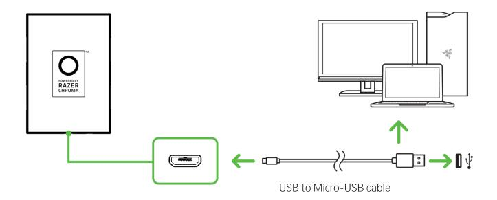
Step 1: Make sure that the Razer Chroma HDK is connected to your PC using the included USB to Micro-USB cable.
